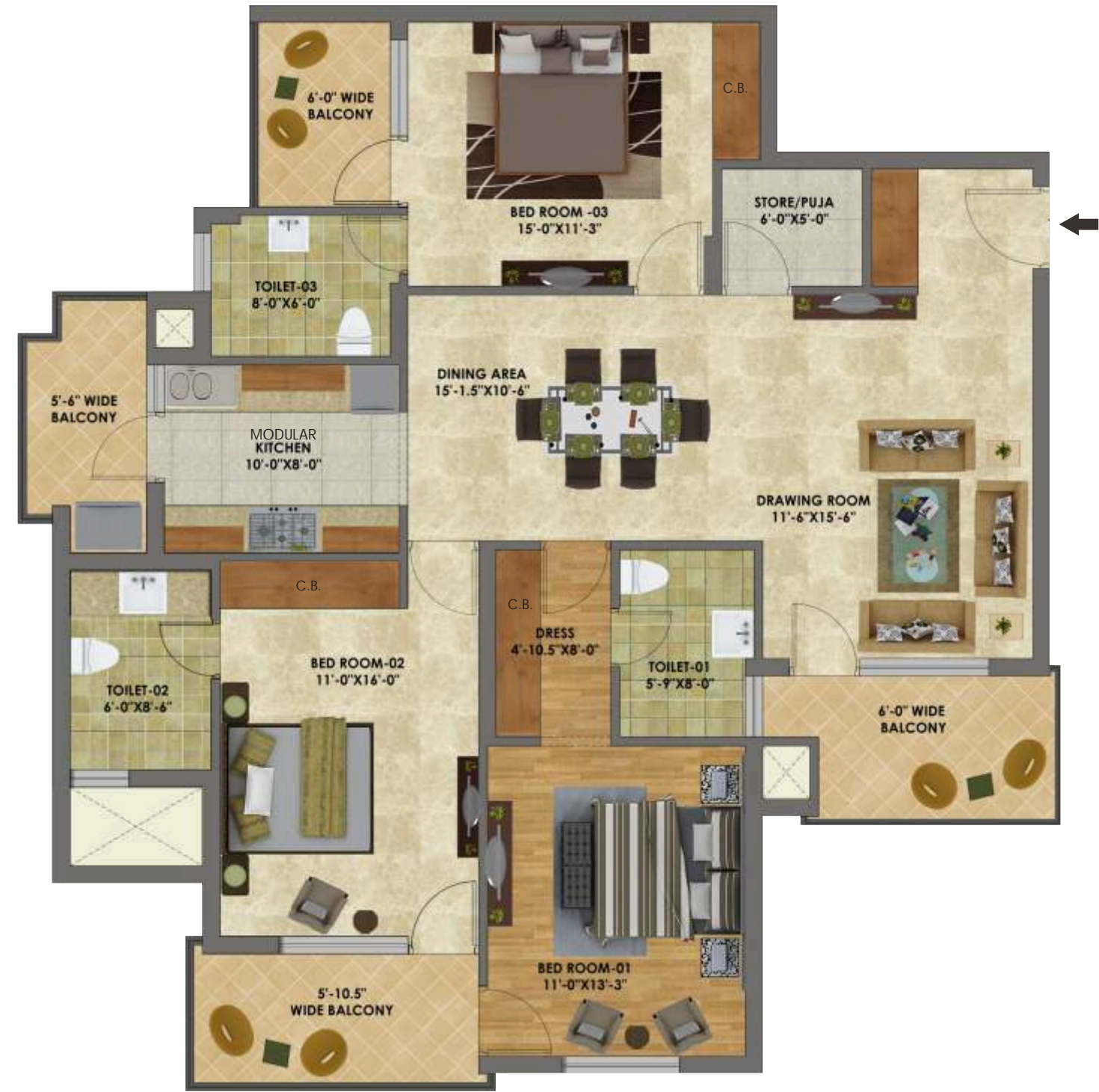
Layout Plan - 'Platinum' 3 BHK (3B+3W), Super Area - 1685 sq.ft. (Super Area Excluding Car Parking Area)
